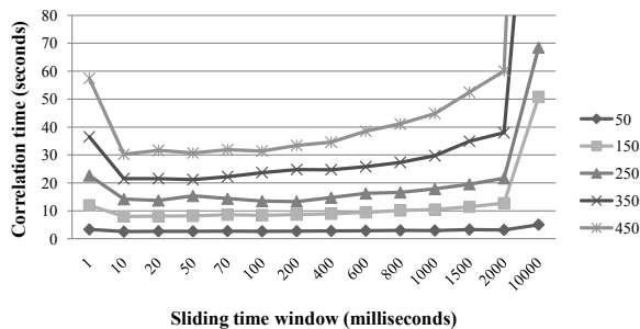
Fig. 15. The partially enlarged view of the correlation time v.s. the size of the sliding time window.
