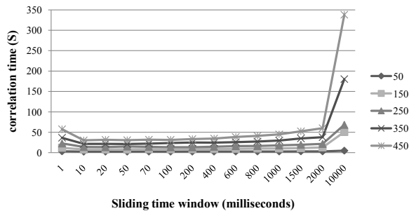
Fig. 14. The correlation time v.s. the size of the sliding time window. The concurrent clients varies from 50 to 450.
